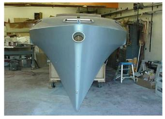
But if there's a knuckle being used, this seldom happens, especially when combined with an overhanging deck. Just compare a Dragonfly 25/800 with an F25 and you'll soon notice the difference. Both hulls are just over 25' long.
