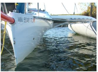
with a thin skin of it on each side of a semi-rigid foam. There's no doubt that this can produce a lighter and more rigid panel than even one of plywood, but at what cost? Not only is the production and material cost high but also the thin exterior skin remains fragile against sharp objects.
